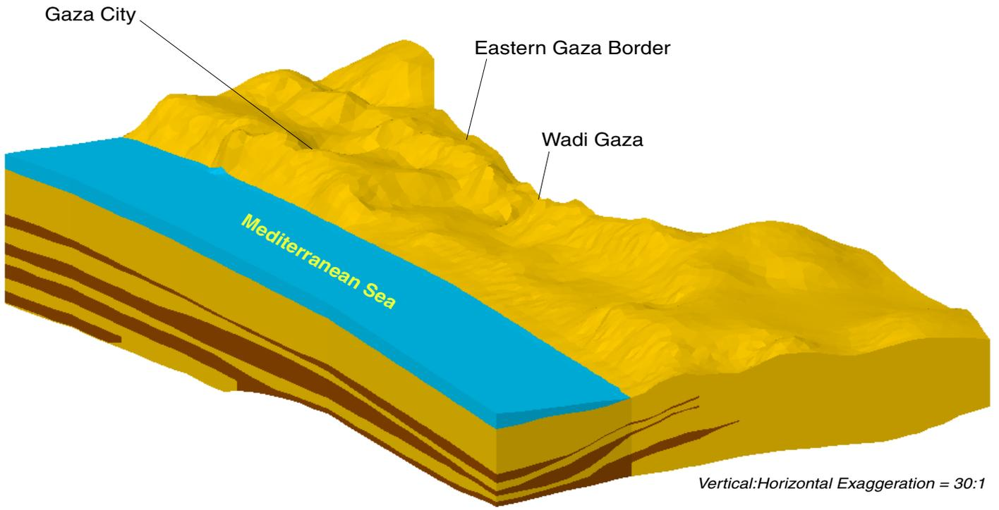
**Figure 2:** Model Topography and 3-D View of Stratigraphy, Gaza Strip
