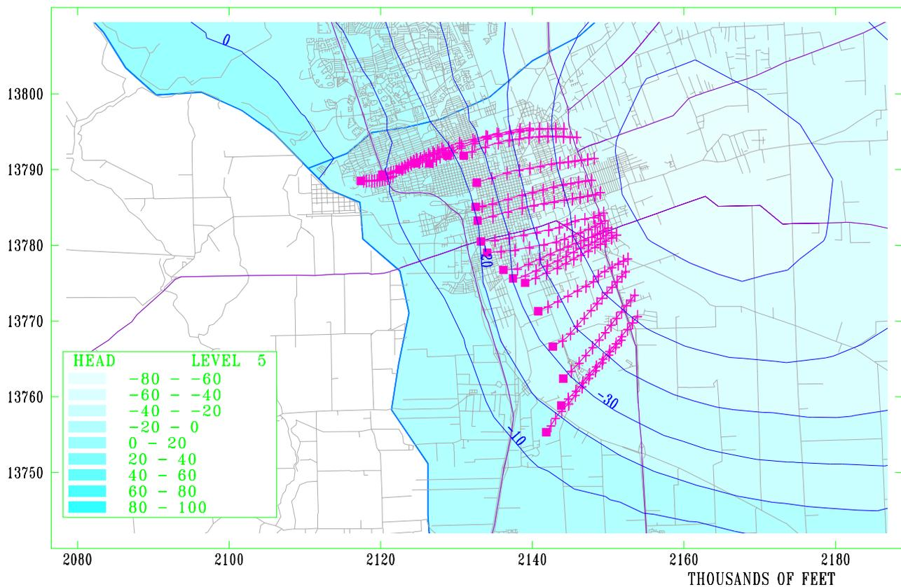
**Figure 7:** Simulated Particle Tracks (60 Years, 5 Year Intervals)
