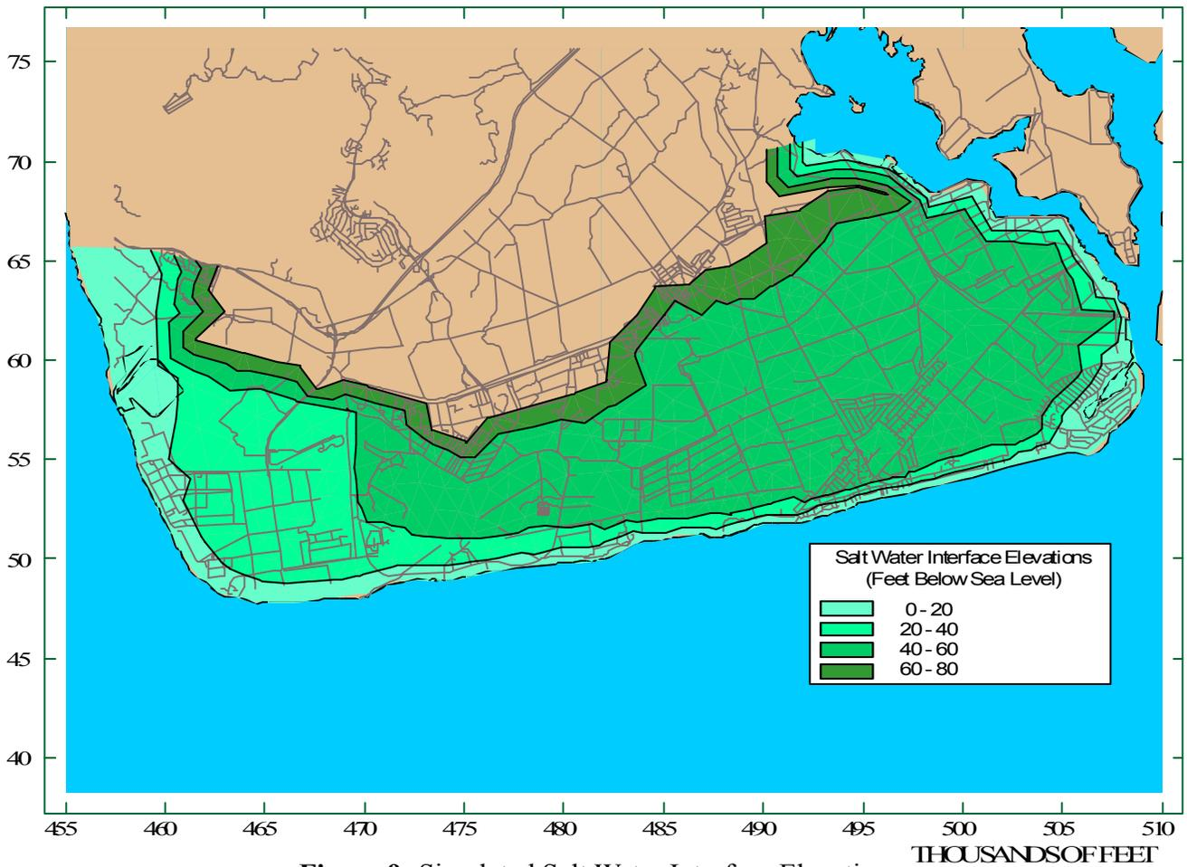
**Figure 9:** Simulated Salt Water Interface Elevations
