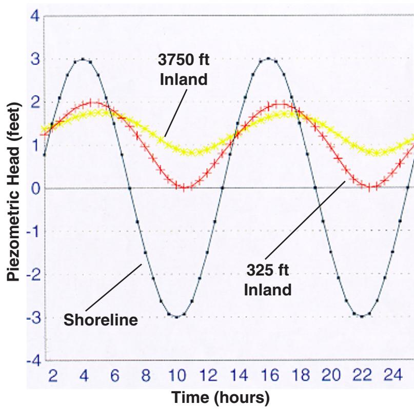
**Figure 8:** Simulated Tidal Response
