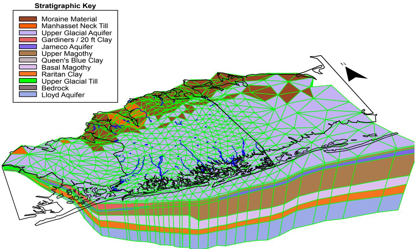
**Figure 3:** 3-D View of Model Grid and Stratigraphy, Long Island, NY
