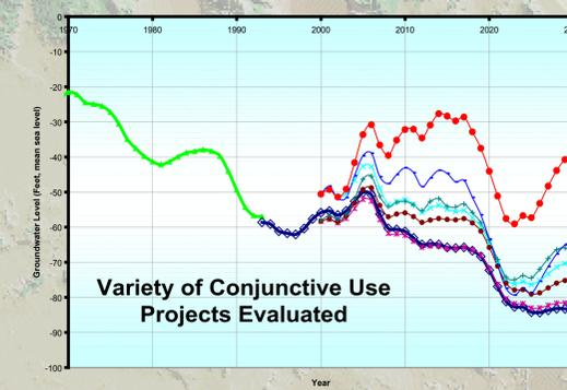
Simulate conjunctive use alternatives to assess benefits in terms of increasing groundwater levels, and rate of lateral intrusion.
