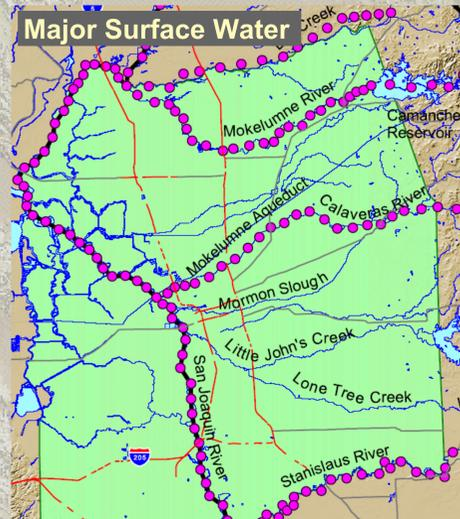
Surface water is hydraulically connected to groundwater in the Eastern San Joaquin Basin. Groundwater pumping significantly impacts surface water availability and operations. Thus, in addition to the familiar groundwater model parameters, a sufficient level of detail in surface water hydrology and landuse must be incorporated into the model.
